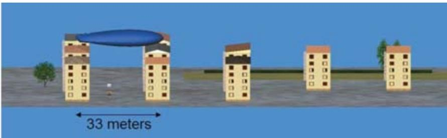
**Figure 5.** The compliance distance of a typical roof-mounted base station, calculated for an exposure limit of 0.6 V/m, is 165 meters in the forward direction.<sup>5</sup>
