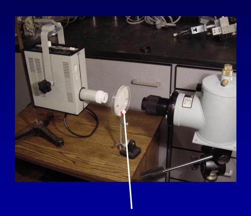
Phantom- 0.2 mm thick saline saturated filter paper absorber
