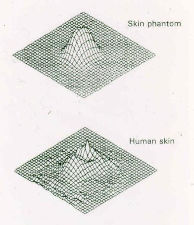
Heating patterns resulting from mm-wave irradiation from the open side of a rectangular waveguide under similar exposure conditions
