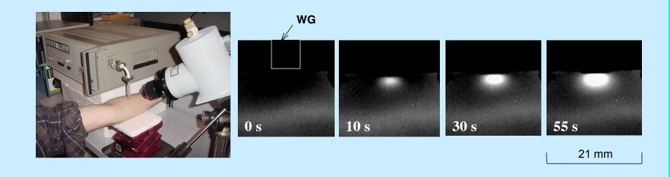
IR images show the forearm skin at 0, 10, 30, and 55 s following exposure with the WG ( $I_o = 208 \text{ mW/cm}^2$ ). The distance between the open end of WG and skin surface was 2.5 mm. The lighter band on the bottom of each thermogram corresponds to the warmer skin area located above a vein. Baseline skin temperature was 32.5 °C. Maximum temperature at 55 s was 35.7 °C.
