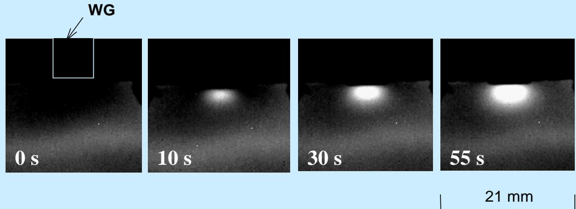
IR images show the forearm skin at 0, 10, 30, and 55 s following exposure with the WG ( $I_0 = 2080 \text{ W/m}^2$ ). The distance between the open end of WG and skin surface was 2.5 mm. The lighter band on the bottom of each thermogram corresponds to the warmer skin area located above a vein. Baseline skin temperature was 32.5 °C. Maximum temperature at 55 s was 35.7 °C.
