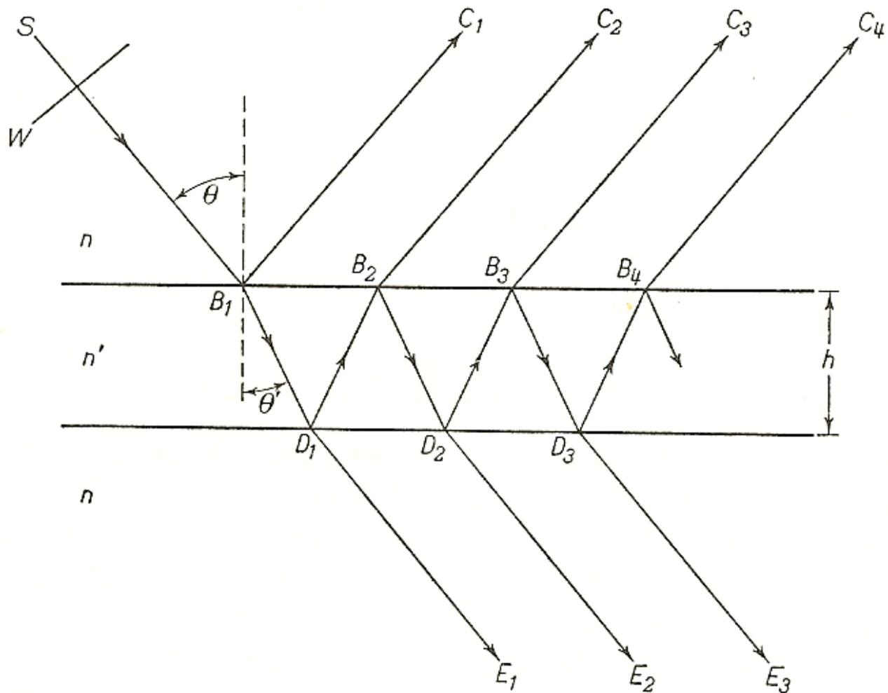
Fig. 7.56. Reflection of a plane wave in a plane parallel plate.
